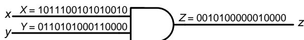
Figure 2. AND gate as a stochastic multiplier, with p_x = 8/16 , p_y = 6/16 and p_z = p_x \times p_y = 3/16 . Equivalently, Z = X \times Y = 3/16 .
