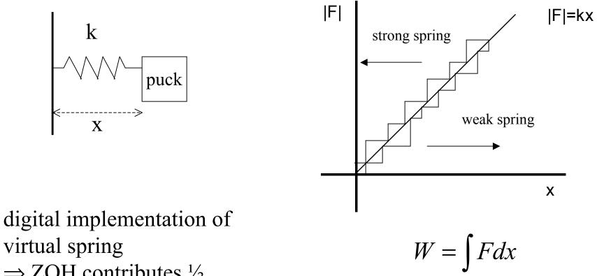
$\Rightarrow \text{ZOH contributes } \frac{1}{2}$ sample delay  $\Rightarrow \text{spring adds energy}$
