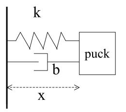
Equivalent to adding damping b = kT/2 to the virtual wall
