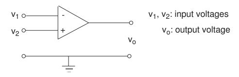
• output voltage depends on *difference* of input voltages
