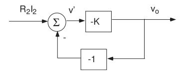
• Apply rule for transfer function of feedback system:
