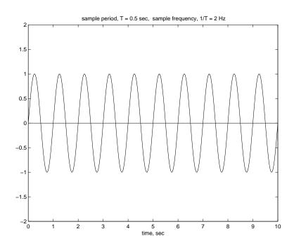
• Input: a 1 Hz sinusoid,  $\sin(2\pi t)$ , sampled at 1.11 Hz
