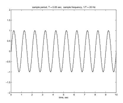
• Input: a 1 Hz sinusoid,  $\sin(2\pi t)$ , sampled at 10 Hz
