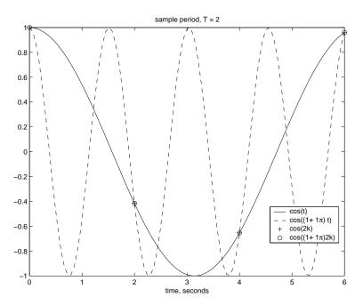
• A higher frequency signal that "masquerades" as a low frequency signal after sampling is said to be *aliased*.
