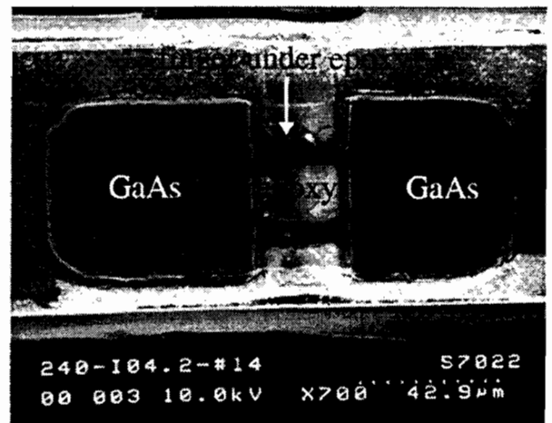
Figure 7: SEM photo of a device without AlGaAs layer, after 240°C lifetime test. This device degraded gradually, and shows no sign of cracks in the GaAs mesas.
