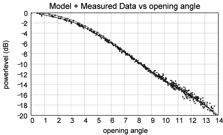
Figure 4 Comparison of model and experimental data of a band 3 horn at 893 GHz
