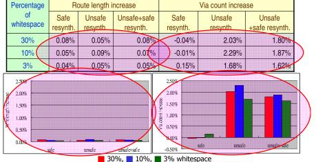
Route length increase is small for all layouts, while via count increase is significant for layouts produced by unsafe resynthesis 23
