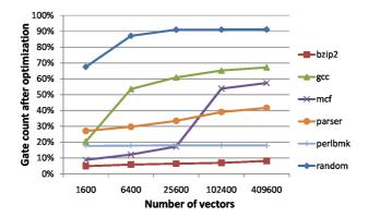
Fig. 7. Gate count after specializing the Alpha CPU with SignalMerge. 30-90% of the gates can be removed for applications as long as half-million dynamic instructions.
