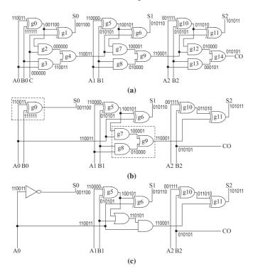
Fig. 5. Ripple-carry adder specialization example: (a) original circuit, (b) after SignalMerge, and (c) after ShannonSynth. Allowed input values are 3, 4, 5 (for A) and 1 and 7 (for B).
