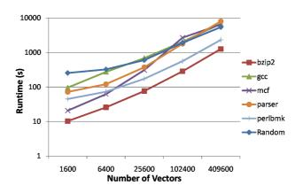
Fig. 8. SignalMerge runtime to specialize Alpha. Runtime is approximately linear on the number of stimulus vectors used.
