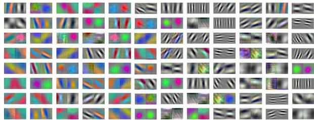
Figure 1. Visualization of conv1 filters from AlexNet. Each filter and its pairing filter ( $w_i$  and  $\bar{w}_i$  next to each other) appear surprisingly opposite (in phase) to each other. See text for details.
