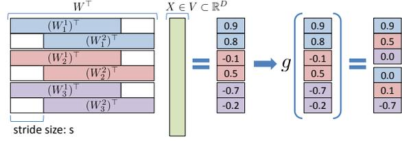
Figure S1. An illustration of convolution, CReLU, and max-pooling operation. For simplicity, we describe with 3 convolution filters ( $W_1, W_2, W_3$ ) with stride of  $s$ , and with  $2 \times 2$  pooling. In Figure (a),  $g$  denotes CReLU followed by the max-pooling operation.
