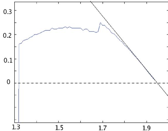
Fig. 2. Inverse sensitivities for a power system example. The  $x$ -axis represents the fault-clearing time, while the  $y$ -axis is the inverse sensitivity of the response time. The inverse sensitivity has an affine dependence on the disturbance parameter, with slope equal to roughly  $-1.2$  (as indicated by the straight line in the plot).
