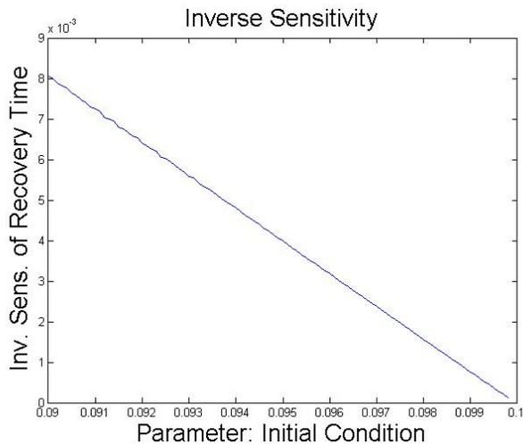
Fig. 1. A nonlinear model for virus-spread control is considered. The inverse sensitivity of the recovery time to a virus-free state with respect to the initial infection fraction is shown. For initial conditions near the critical point (unstable equilibrium), the inverse-sensitivity is affine with respect to the initial condition with slope 0.8, as predicted.
