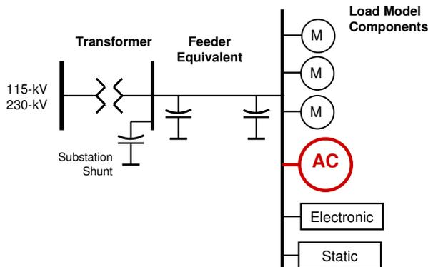
Figure 1: WECC load model structure.
