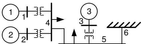
**Fig. 1 - Single-line diagram of the 3MIB system**
