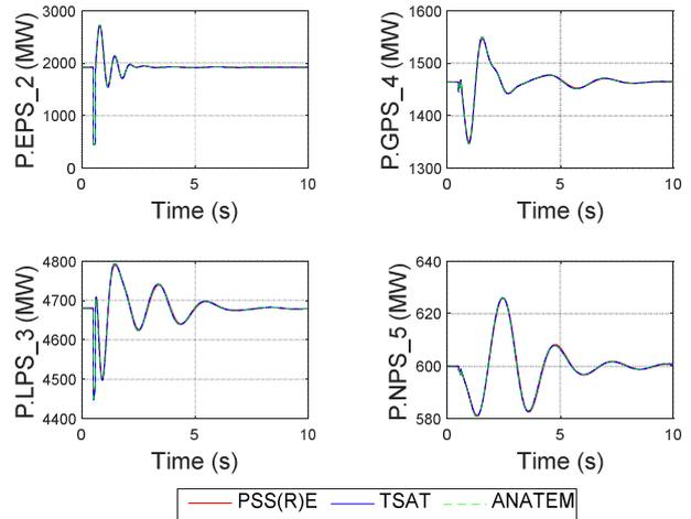
Fig. 14 – 14-gen system, case 2: Comparison of generator power outputs with two-phase to ground fault applied to bus 209.
