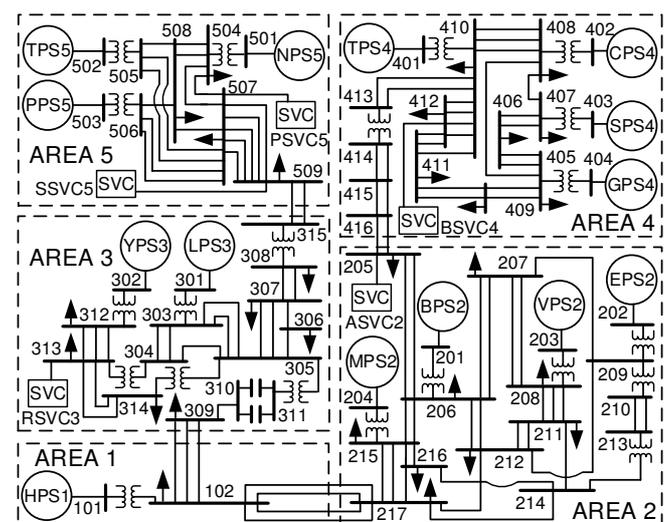
**Fig. 5 - Single-line diagram of the 14-generator system**
