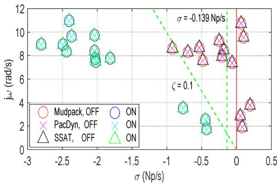
Fig. 13 – 14-generator system, case 2: Comparison of electromechanical modes with PSSs in- (ON) and out-of-service (OFF).
