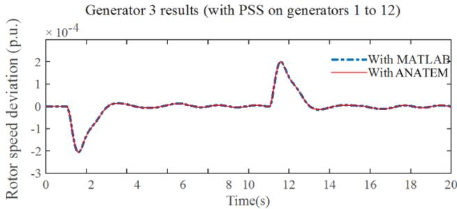
**Fig. 16 – 68-bus system: Nonlinear time-domain simulation results**
