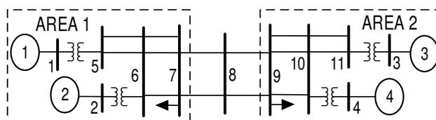
**Fig. 3 - Single-line diagram of the 4-generator system**
