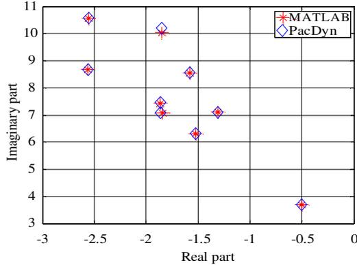
Fig. 12 - 39-bus system: Electromechanical modes (with PSS)
