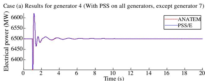
Fig. 10 – 7-bus system: Simulation results for case (a).
