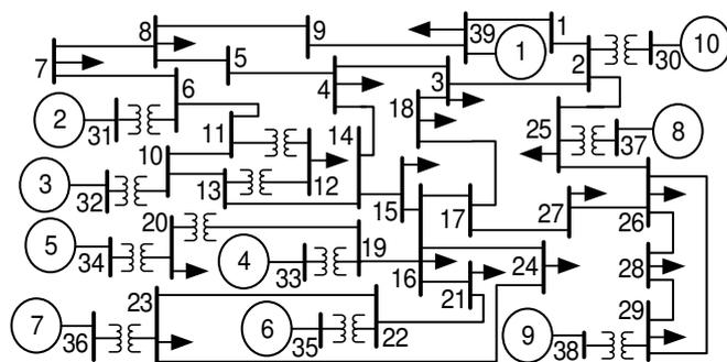
**Fig. 4 - Single-line diagram of the 39-bus system**
