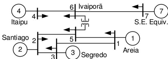
**Fig. 2 - Single-line diagram of the 7-bus system**
