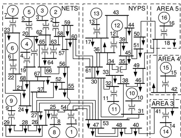
Fig. 6 - Single-line diagram of the 68-bus system
