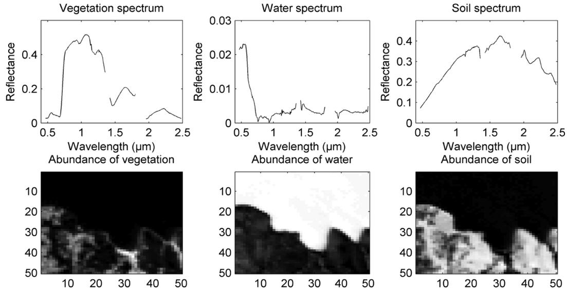
Fig. 8. Top: the  $R = 3$  endmember spectra estimated by the algorithm in the Moffett Field scene. Bottom: the corresponding abundance maps (black (respectively, white) means absence (respectively, presence) of the material).
