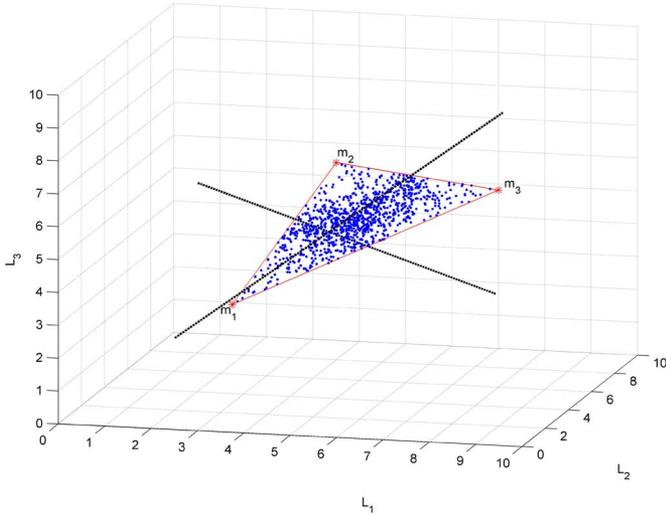
Fig. 2. Example of hyperspectral data observed in 3 spectral bands. The mixed pixels (blue points) belong to the  $R$ -dimensional convex polytope  $\mathcal{S}_M$  (red lines) whose vertices are the endmembers spectra  $\mathbf{m}_1, \dots, \mathbf{m}_R$  (red stars). The first two principal axes estimated by a PCA appear in dashed lines and define the projection subset  $\mathcal{V}_K$ .
