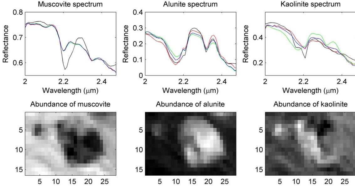
Fig. 10. Top: the  $R = 3$  endmember spectra estimated by the Bayesian (red lines), N-FINDR (blue lines) and VCA (green lines) algorithms in the Cuprite scene, compared with the signatures extracted from the USGS spectral library (black lines). Bottom: the corresponding abundance maps estimated by the Bayesian algorithm (black (respectively, white) means absence (respectively, presence) of the material).
