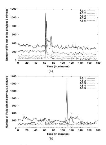
Figure 7: (a) A sharp increase in number of clients lost is seen in all ASes indicating a problem with the server (b) A sharp rise in number of clients lost is seen in a single AS indicating a problem in that AS
