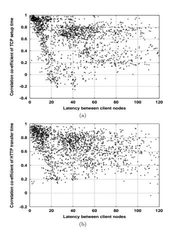
Figure 6: Spatial stationarity of (a) TCP connection setup time and (b) HTTP transfer time: Both show strong correlation when client nodes are within 20 ms of each other.
