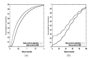
Figure 10: Distribution of delays as observed by the application and by the DSMI for making DNS lookup measurements based on data from (a) gs1 and, (b) gs2 and gs3
