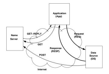
Figure 1: Basic architecture of ATMEN
