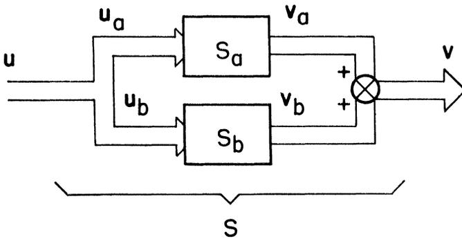
FIG. 2. Parallel connection of  $S_a$  and  $S_b$ .
