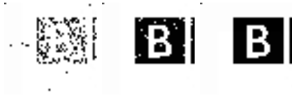
Figure 8: Stealing a 48 \times 48 pixel region from www.bbc.com , at 100 \times 100 , 200 \times 200 , and 300 \times 300 pixel-inspection div size.
