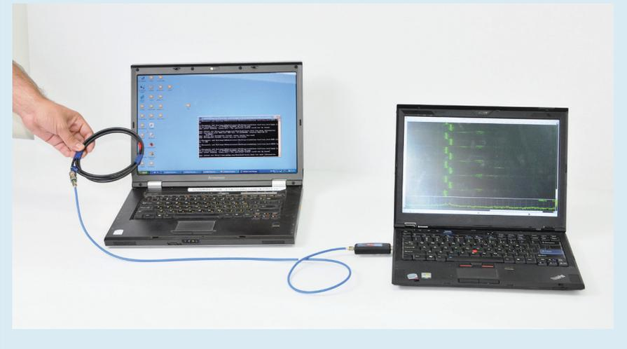
**Figure 10. Extracting keys by measuring a laptop’s electromagnetic emanations through a PITA device.**
