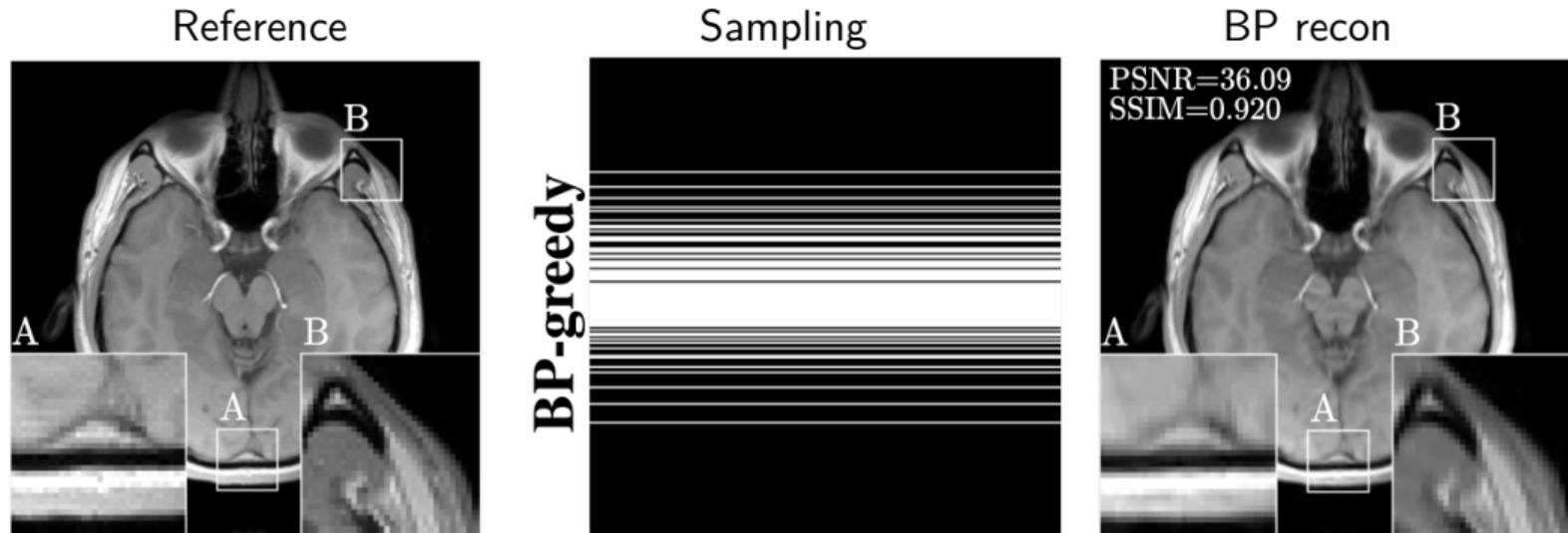
Sampling designed to optimize PSNR for basis pursuit (BP) reconstruction using shearlet transform, at 25% sampling rate.
