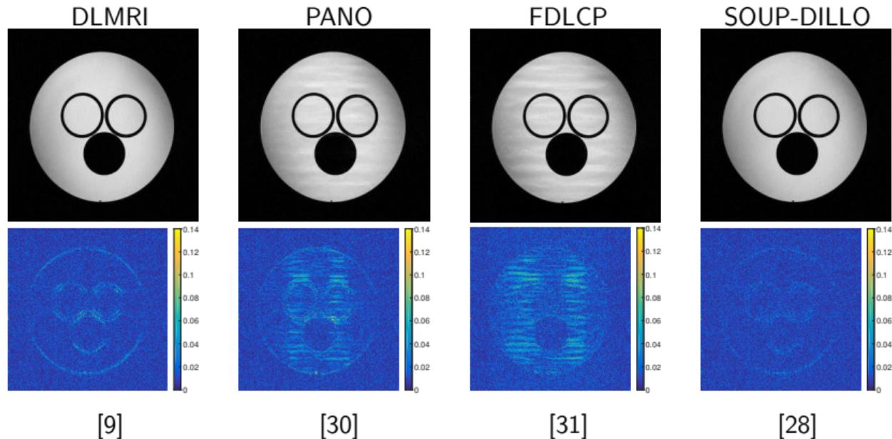
Summary: 2D static MR reconstruction from under-sampled data with adaptive dictionary learning and convergent algorithm, faster than K-SVD approach of DLMRI.
