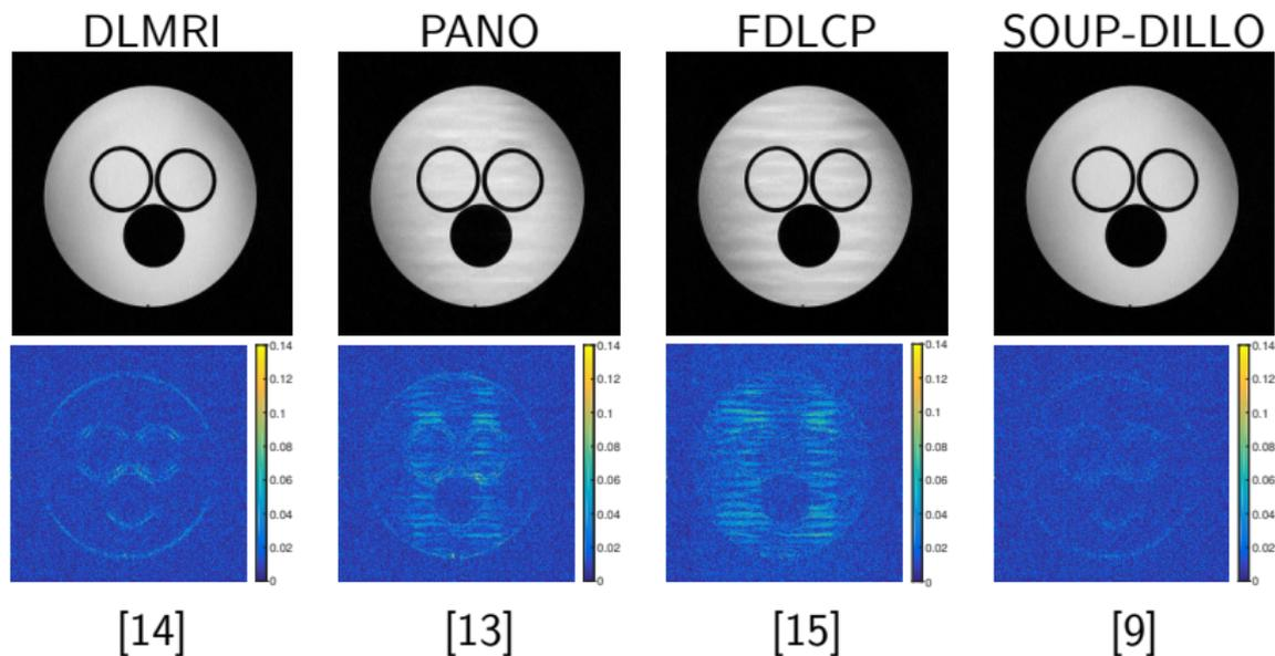
Summary: 2D static MR reconstruction from under-sampled data with adaptive dictionary learning and convergent algorithm, faster than K-SVD approach of DLMRI.
