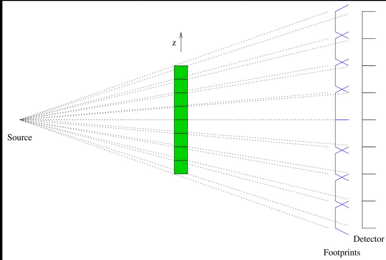
Typically the axial footprints of 2-3 voxels overlap on any given detector cell. Amount of overlap depends on magnification factor.
