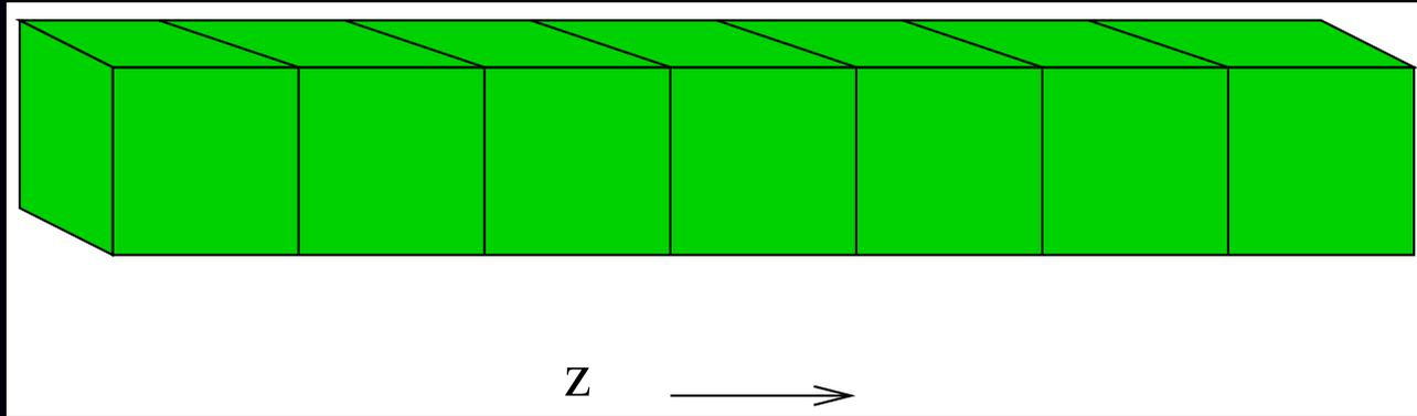
3D regularizer couples each voxel in an axial block to two adjacent voxels. (One in the slice above, one in the slice below.)
