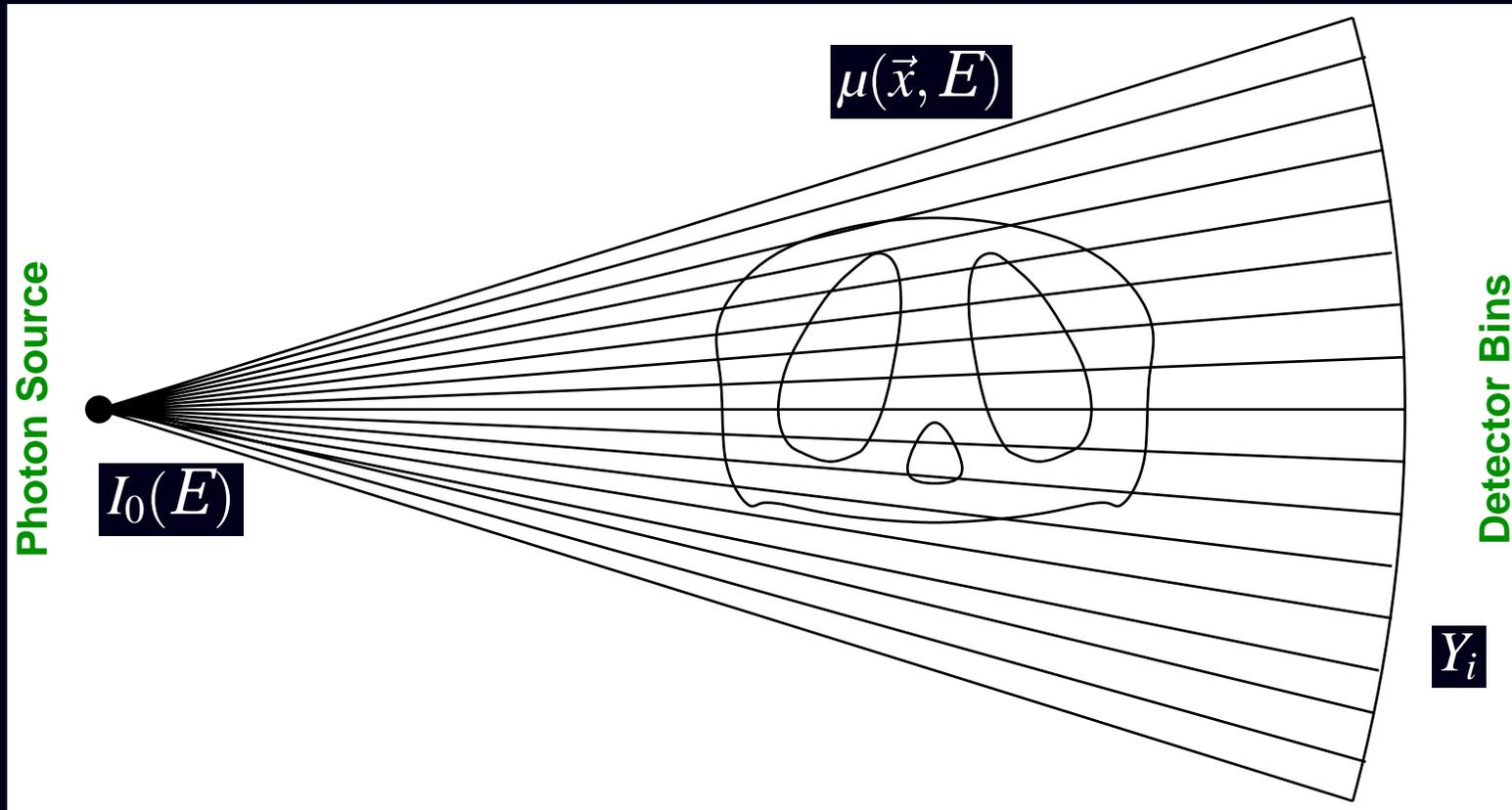
Transmission scanning geometry.
