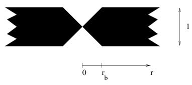
Figure 3. Profile through an approximate Laplacian pinhole.
