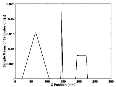
Figure 4. Sample means of 4000 realizations of the estimates of  $\lambda(x)$ , for 21 Gaussian pinhole sizes ranging from 0.9 to 2.9 mm FWHM. The 21 mean curves are virtually indistinguishable since the reconstructed spatial resolution has been held fixed at 3mm FWHM.
