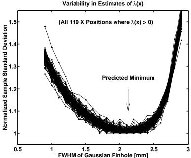
Figure 6. Normalized sample standard deviations of 4000 realizations of the estimates of  $\lambda(x)$ , versus the FWHM of the Gaussian pinhole sizes. There are 119 plots, one for each of the x positions for which  $\lambda(x) > 0$ . The minimum is consistently near the theoretical prediction of  $3/\sqrt{2} \approx 2.1$ .
