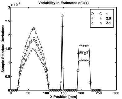
Figure 5. Sample standard deviations of 4000 realizations of the estimates of  $\lambda(x)$ , for 3 of the 21 Gaussian pinhole sizes: 1, 2.1, and 2.9 mm FWHM.
