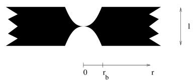
Figure 1. Profile through an approximate Gaussian pinhole.
