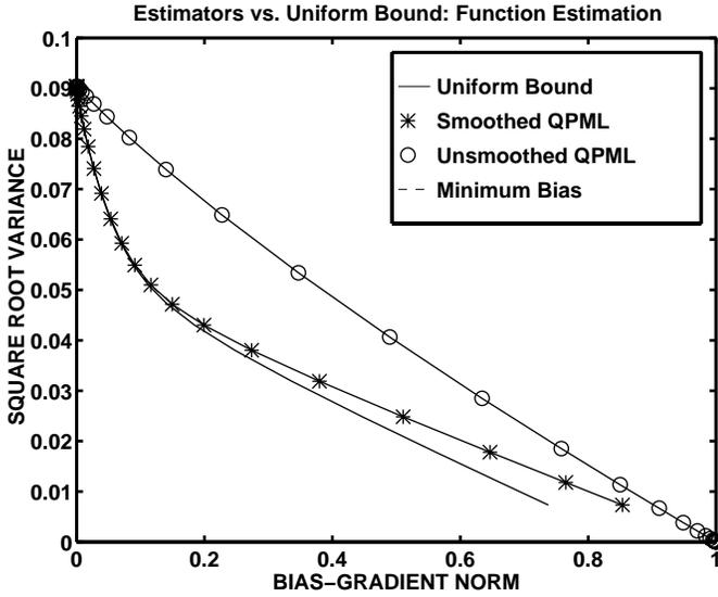
Fig. 7. Bias variance tradeoff study for estimation of nullspace compound  $\underline{h}^T \underline{\theta}$  for singular Fisher information ( $\underline{h}$  is illustrated in Fig. 6). The bound is exactly achieved by the smoothed QPML estimator at the point  $\delta = 5.4 \times 10^{-6}$ .
