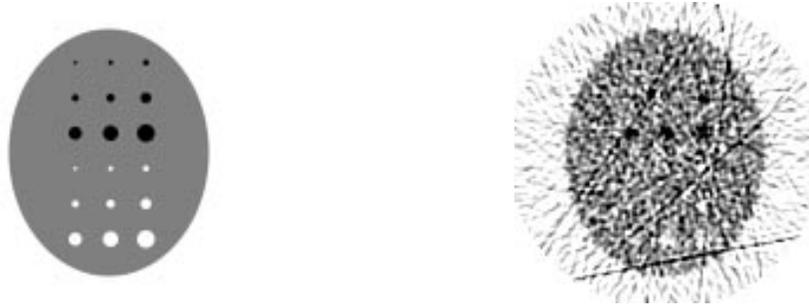
Figure 3: Left: ideal emission distribution. Right: ramp-filtered CBP reconstruction from 600K event scan.
