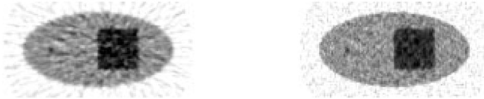
Figure 9: Typical attenuation image reconstructions, left: 3rd order Butterworth with cutoff frequency 40% of Nyquist, right: spline-smoothed with  $\beta = e^2$ .
