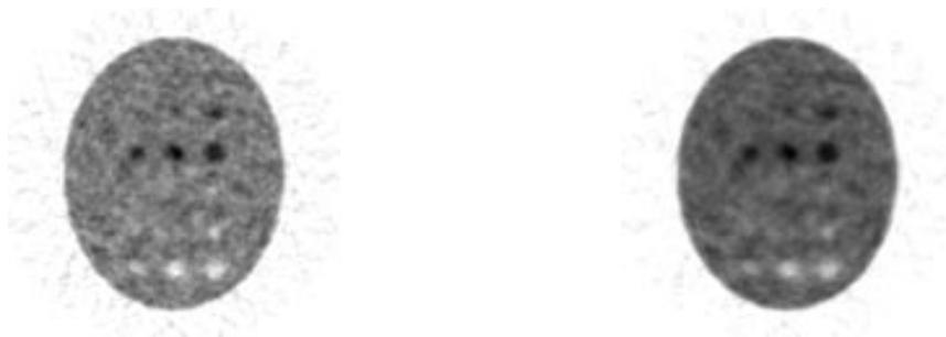
Figure 7: As above but with larger smoothing parameters: left:  $\beta = e^{-6}$ , right:  $\beta = e^{-5}$ . Note the absence of streak artifacts and the different noise structure.
