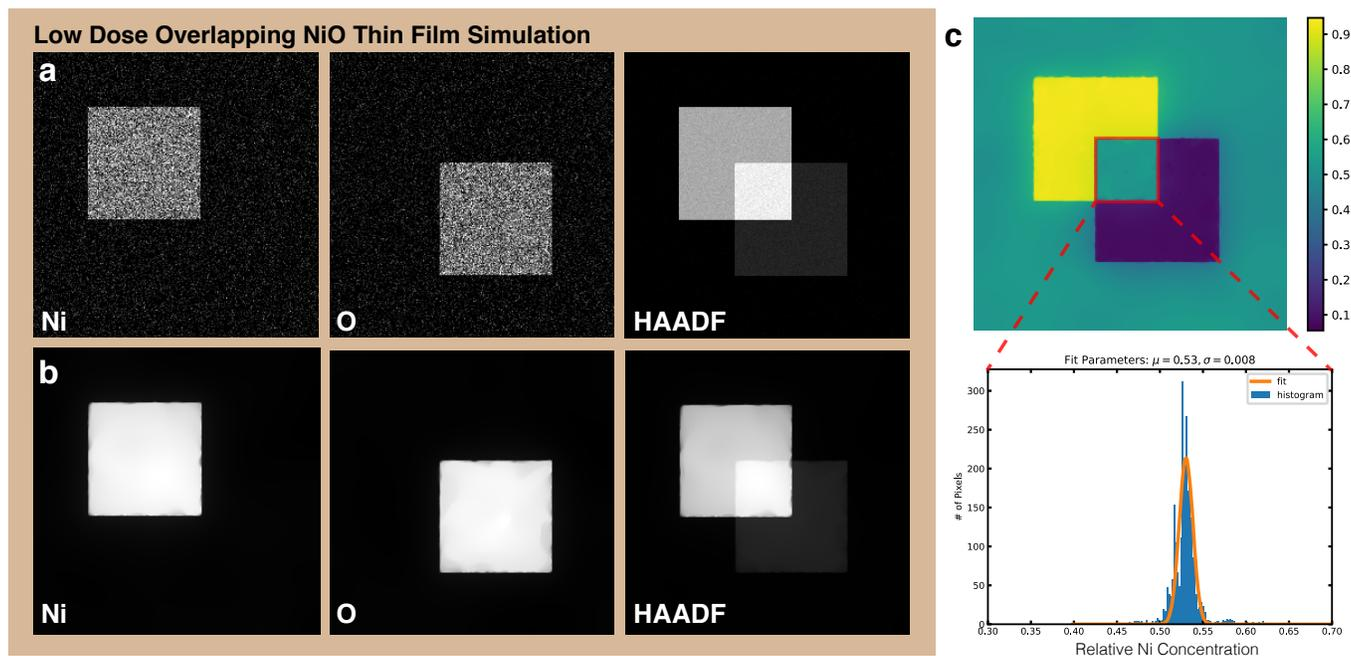
**Supplementary Figure 12** | a-b) Simulated and reconstructed Nickel, Oxygen and HAADF micrographs with concentrations inspired the experimental sputtered thin film. At low electron doses, TV regularization is unable to maintain the sharp edges. c) Ni ratio map and histogram of the overlapping region (indicated in red), the average concentration is  $\sim 53\%$ .
