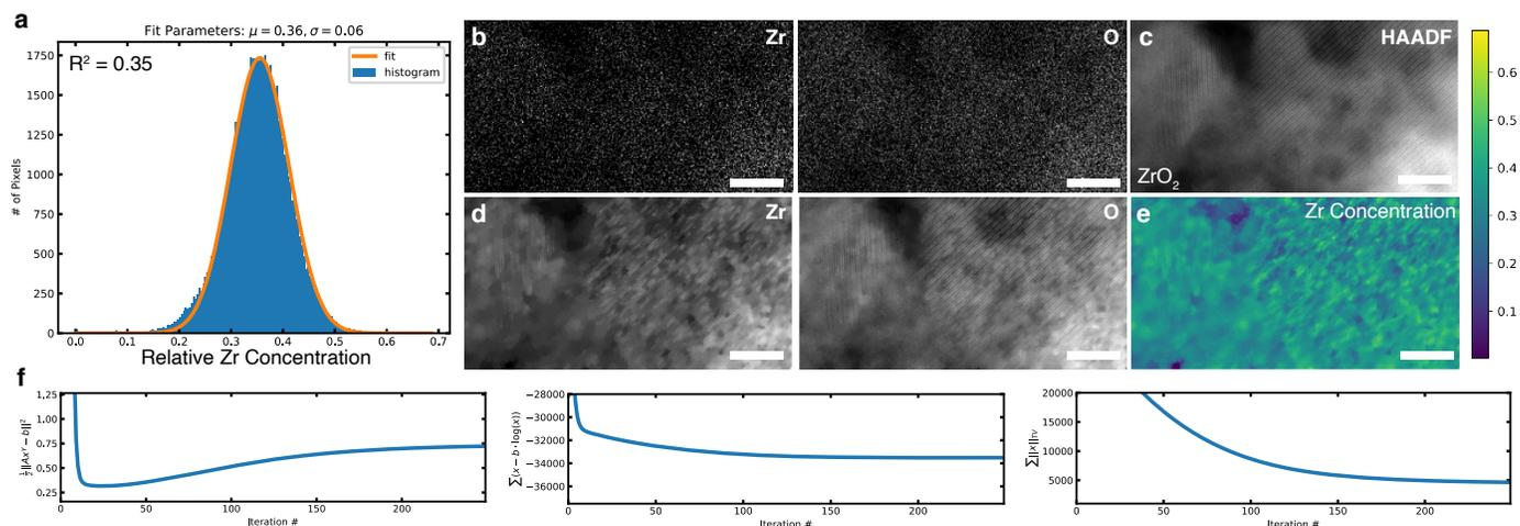
**Supplementary Figure 8 |** a) Histogram of intensities for the Zr distribution for a sputtered ZrO<sub>2</sub> thin film. The fit parameters and  $R^2$  values for this Gaussian are reported. b-c) The raw EDX maps and simultaneous HAADF for the Zr and Oxygen distribution. d-e) The multi-modal reconstructions for the constituent elements and Zr concentration map. f) Convergence plots for each term in the cost function. Scale bar, 5 nm.
