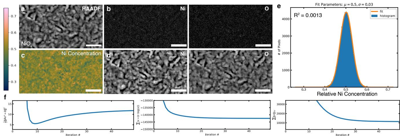
**Supplementary Figure 9 |** a-b) The raw EDX maps and simultaneous HAADF for the nickel and oxygen distribution. c-d) The multi-modal reconstructions for the constituent elements and Ni concentration map. e) Histogram of intensities for the Ni distribution for a sputtered NiO thin film. The fit parameters and  $R^2$  values for this Gaussian are reported. f) Convergence plots for each term in the cost function. Scale bar, 20 nm.
