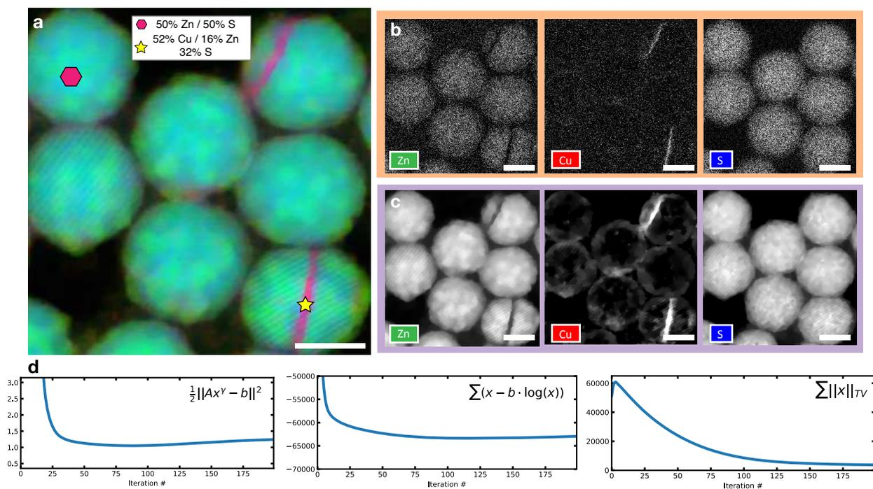
**Supplementary Figure 4** | a) An RGB chemical overlay for the Zn, Cu, and S distributions. The two points labeled in the white box reports concentrations for the three elements. b-c) The raw EELS maps and multi-modal reconstructions. d) Convergence plots for the three components in the cost function: model based term, data fidelity, and regularization. Scale bar, 10 nm.
