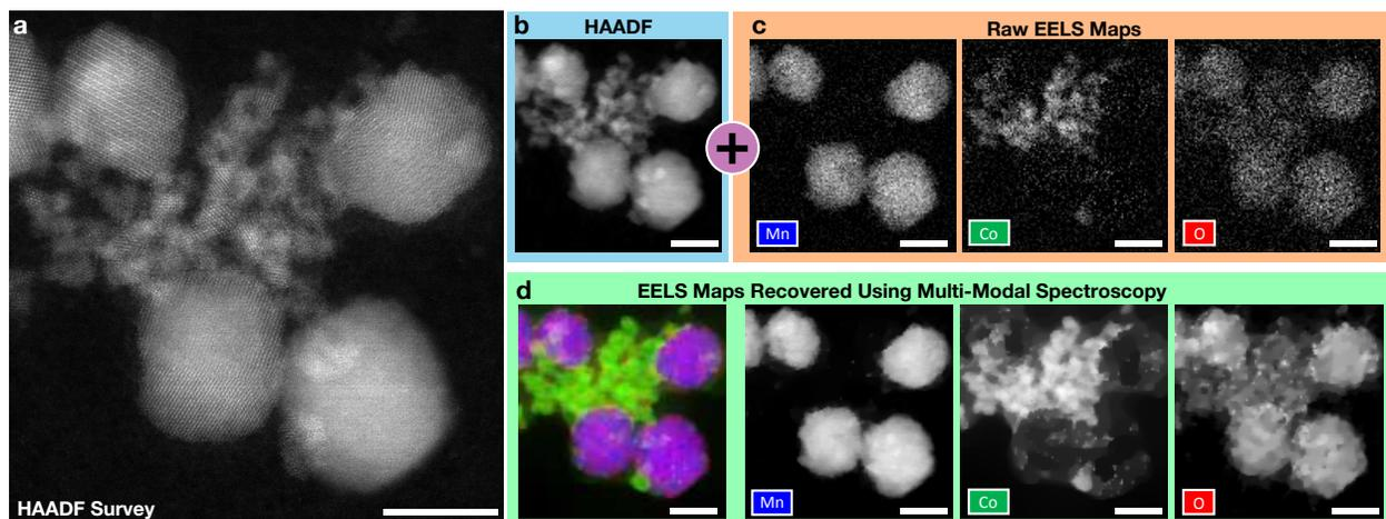
**Supplementary Figure 3** | a) HAADF survey image of the nanoparticles confirming that both the  $\text{CoO}$  and  $\text{MnO}$  nanoparticles are indeed crystalline. b-c) The simultaneous HAADF and raw EELS maps of the nanoparticles. d) An RGB chemical overlay and constituent recovered maps for Mn, Co, and O distributions. Scale bar, 5 nm.
