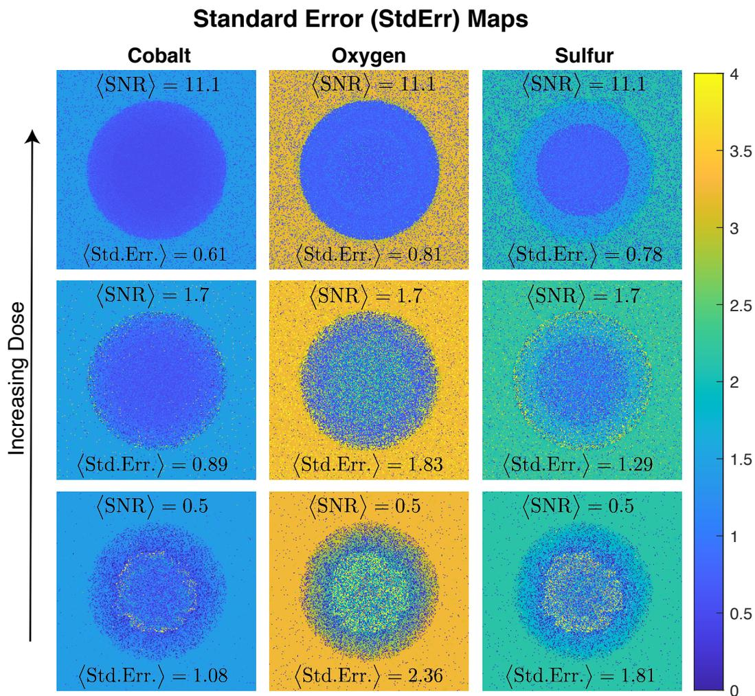
**Supplementary Figure 10** | Visualization of the standard error (StdErr) maps for the synthetic CoS core shell simulation in Fig. 6b. As we increase the electron dose, the average StdErr pixel values for all three elements decreases.  $\langle \text{SNR} \rangle$  denotes the average SNR between the chemical and HAADF modality.
