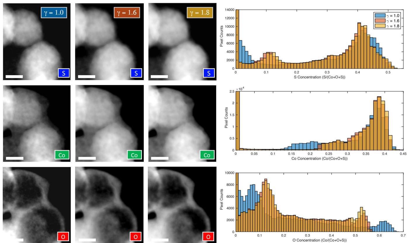
**Supplementary Figure 6** | Histogram of intensities for the Sulphur, Cobalt and Oxygen distributions when  $\gamma$  varies between 1.0, 1.6, and 1.8. We see for values close to 1.7, the specimen's relative concentrations almost perfectly matches the distribution in Fig. S5. However if gamma is far off from what is experimentally feasible ( $\gamma = 1.0$ ), the measured concentrations are incorrect. Scale bar, 30 nm.
