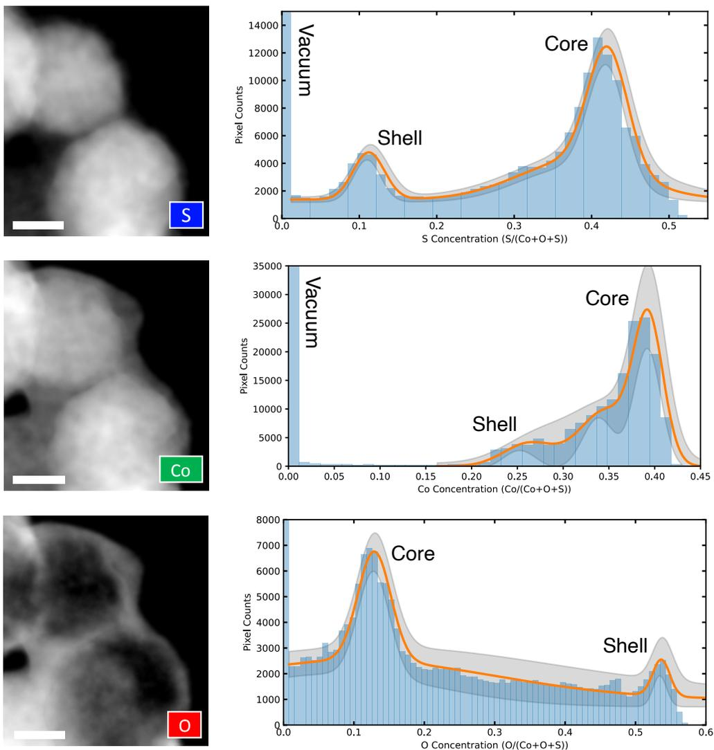
**Supplementary Figure 5 |** Histogram of intensities for the Sulphur, Cobalt and Oxygen distributions. Due to the core-shell structure consisting of two phases, the histograms contain of two Gaussian distributions. The specimen core contains a relative concentration of  $39 \pm 1.6\%$ ,  $42 \pm 2.5\%$  and  $13 \pm 2.4\%$  and exterior shell composition of  $26 \pm 2.8\%$ ,  $11 \pm 2.0\%$ ,  $54 \pm 1.3\%$  for Co, S, O respectively. Scale bar, 30 nm.
