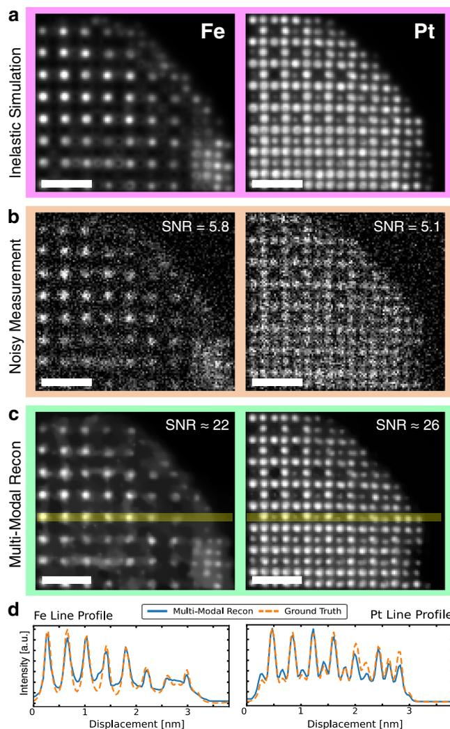
**Fig. 4 Inelastic FePt nanoparticle simulation.** **a** Ground truth EELS images generated from inelastic simulations. **b** EELS maps degraded with Poisson shot noise. SNR is shown on the top right. **c** Recovered atomic-resolution EELS maps for the Fe and Pt distributions. Estimated SNR is shown on the top right. **d** Line profiles of the marked yellow bars (10 pixels in width) in (c) compares the multi-modal reconstruction and ground truth. Scale bar, 1 nm.
