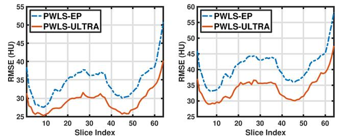
Fig. 6. RMSE of each axial slice in the PWLS-EP and PWLS-ULTRA reconstructions for  $I_0 = 1 \times 10^4$  (left) and  $I_0 = 5 \times 10^3$  (right).
