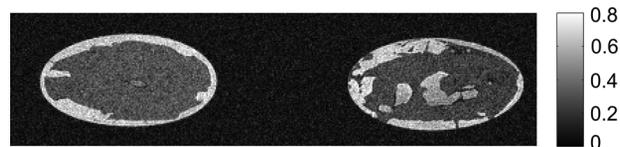
Fig. 8. Magnitude of the breast phantom body coil image.
