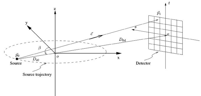
Fig. 1. Axial cone-beam flat-detector geometry.
