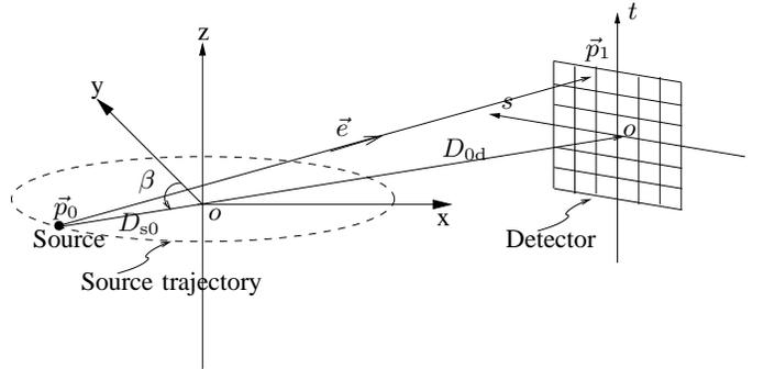
Fig. 1. Axial cone-beam flat-detector geometry.
