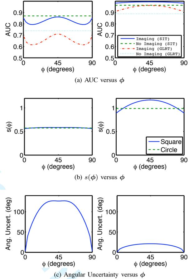
Fig. 5: AUC, relative sensitivity, and angular uncertainty for square position-sensitive and circular counting detectors of equal area ( $r = 2l/\sqrt{\pi}$ ) vs.  $\phi$  with  $\mu l = 0.5$  (left) and  $\mu l = 5$  (right), and  $\alpha\tau = \lambda_b\tau = 10$ .
