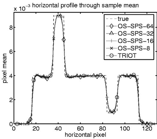
Fig. 7. Horizontal profiles through sample mean of different ordered subsets methods along the dotted line in Fig. 6.
