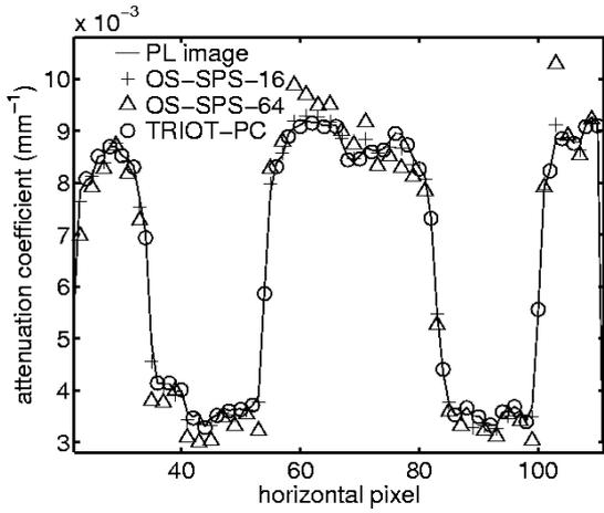
Fig. 5. Horizontal profiles through the PL image in Fig. 4(a), reconstructed attenuation maps for OS-SPS-16 in Fig. 4(c), for OS-SPS-64 in Fig. 4(e), and for TRIOT-PC in Fig. 4(f) along the dotted lines.
