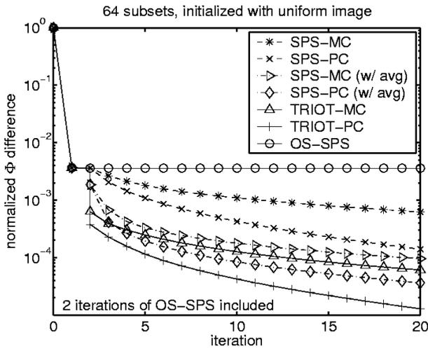
Fig. 3. Comparison of  $(\Phi(\hat{x}^{\text{PL}}) - \Phi(\hat{x}^n)) / (\Phi(\hat{x}^{\text{PL}}) - \Phi(\hat{x}^0))$  versus iteration number. For this figure, 64 subsets are used for OS-SPS and TRIOT algorithms, and two iterations of OS-SPS are included initially for TRIOT and SPS algorithms. This figure also shows the performance of SPS algorithms that include averaging 64 subiterates after 2 iterations of OS-SPS.
