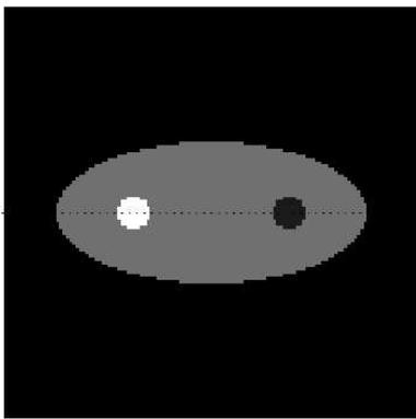
Fig. 6. Digital phantom used in simulation. The background, left hot disc, and right cold disc have attenuation coefficients of  $0.004\text{mm}^{-1}$ ,  $0.009\text{mm}^{-1}$ , and  $0.001\text{mm}^{-1}$ , respectively. Fig. 7 shows the horizontal profiles through the sample mean of ordered subsets methods along the dotted line.
