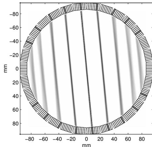
Fig. 5. A space-variant PET system. The above PET system model has physical characteristics chosen to simulate the MicroPET rodent scanner. In the above image, rays connecting every 10th detector are shown. Both nonuniform sampling and varying detector response due to crystal penetration are incorporated in this model.
