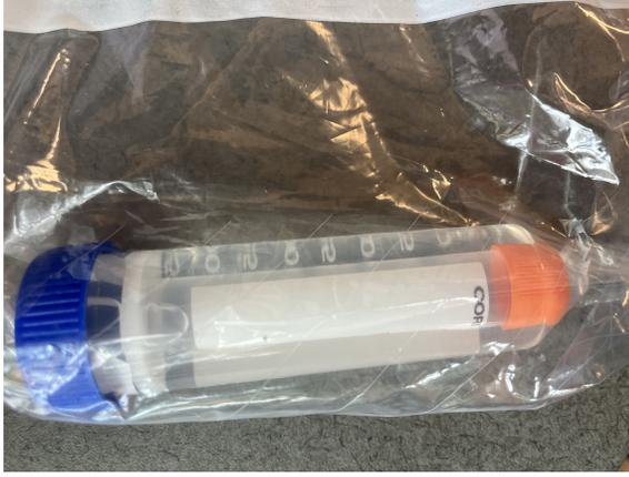
Figure 4.2: Phantom containing urea water solution.
