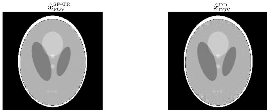
Figure 3.5: Axial views of FOV images  $\hat{x}_{\text{FOV}}^{\text{SF-TR}}$  and  $\hat{x}_{\text{FOV}}^{\text{DD}}$  reconstructed by the iterative method (PWLS-CG) using the SF and DD method respectively. *Left*: SF-TR projector; *Right*: DD projector.
