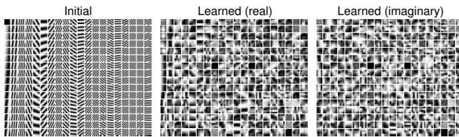
Fig. 11: Dictionaries for the PINCAT data from [60], [61] with 9x undersampling. Left: the atoms of the initial DCT dictionary. Center and right: the real and imaginary parts of the final learned dictionary produced by OnAIR-LD ( $r = 1$ ). The dictionary atoms are  $8 \times 8 \times 5$  tensors, and only the first  $8 \times 8$  ( $x - y$ ) slice of each atom is displayed.
