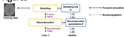
Figure 1. SNOPY learning workflow. The sampling trajectory (and possibly reconstruction parameters) are optimized by gradient-based methods. SNOPY uses differentiable programming to compute the gradients required in the update.
