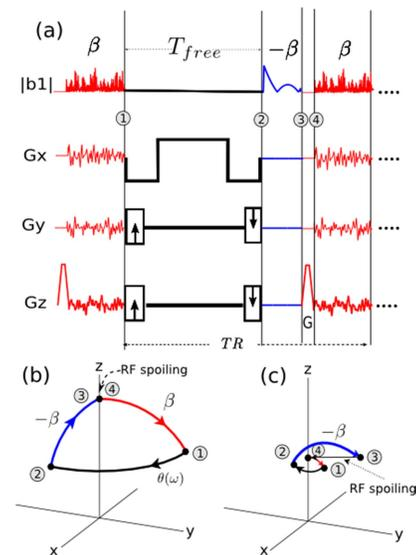
**Figure 1.** Proposed “IVex-STFR” sequence with 3D selective tip-down pulse and spectral pre-winding tip-up pulse. (a) Pulse sequence timing diagram. (b-c) Spin paths for inner volume (IV) and outer volume (OV) regions. The IV region experiences both tip-down and tip-up pulses. The OV region mainly experiences the tip-up pulse. The use of RF spoiling will spoil and partially suppress the steady-state OV signal [2].
