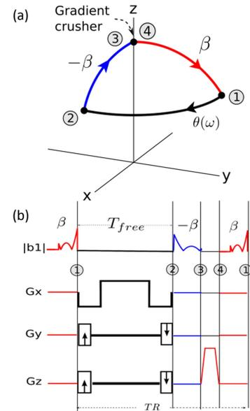
Figure 1. Proposed spectral-STFR pulse sequence. (a) Steady-state spin path. The spin is tipped back to the z-axis by a pulse tailored to the accumulated free precession phase  $\theta = \omega T_{free}$ , where  $T_{free}$  is the free precession time. (b) pulse diagram. Spectral tailored pulses are used for both tip-down and tip-up. Gradient crusher is used without RF spoiling.
