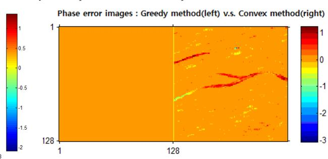
Figure 3. differences in radian between the true  $\theta$  and the estimated  $\theta$  from the greedy method(left) and the convex method(right) with undersampling factor 15
