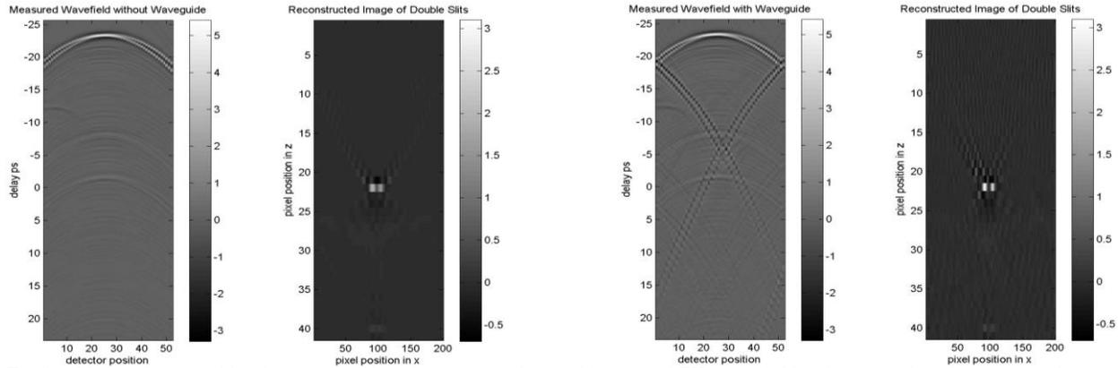
Fig. 2 a) Measured wave field without waveguide and reconstructed image b) measured THz wave field with waveguide and reconstructed image
