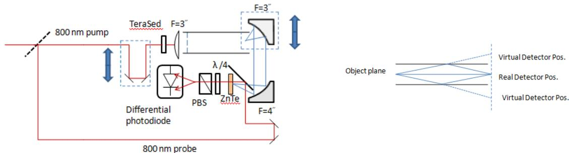
Fig. 1a) The schematic of waveguide THz imaging system 1b) the principle of mirror images as applied to a waveguide
