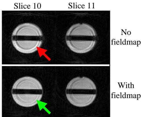
Figure 1: 2 slices of a resolution phantom collected using the 3D FSE. Top two images have no field map in the reconstruction and the bottom 2 include field map.
