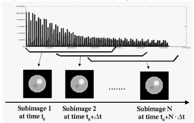
However, the data redundancy in sub-images results in noisy field map estimates. To reduce this error, an iterative method was used as follows: the current estimate of the field map was used to correct susceptibility artifact for each sub-image, then the remaining field map
