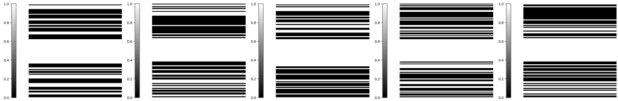
Figure 18: Examples of k -space masks, used in both the fMRI data and the simulated MRI data, where approximately 50% of the pixels are zeroed out, i.e., not measured. These specific masks were used to generate the sub-sampled k -space data for the OSSI dataset, and the masks for the Shepp Logan Phantoms were generated in a similar manner.
