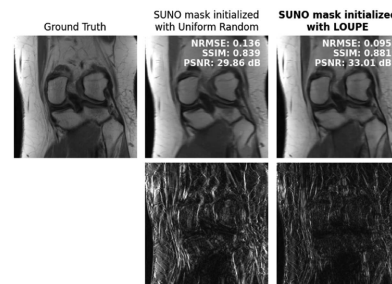
Fig. 9. Comparing reconstructed images using SUNO masks initialized from uniform random and LOUPE masks at 8× acceleration factor.
