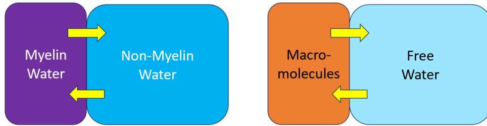
Figure 2.5: Two different two-pool models of white matter. A white matter voxel can be modeled as having a myelin water compartment and a non-myelin water compartment (left). It can also be modeled as having a macromolecular pool and a free water pool (right).
