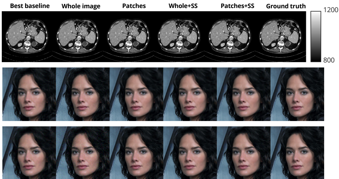
FIG 7.8 – Small dataset setting: Results of inverse problem solving. Top row is 60 view CT recon, middle row is deblurring, and bottom row is superresolution.
