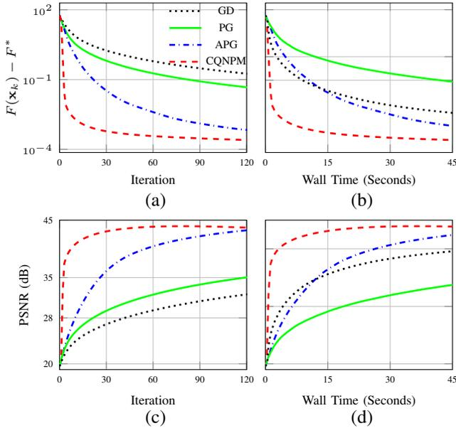
Fig. 5. Comparison of different methods with radial acquisition on the knee image for  $\varepsilon = 8 \times 10^{-5}$ . (a), (b): cost values versus iteration and wall time; (c), (d): PSNR values versus iteration and wall time.
