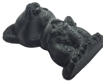
Figure 2: 3D printed reconstruction of the surface you will reconstruct in Problem 8. The 3D printing quality was intentionally set coarse so you can see how the printer constructed the shape from its level curves.
