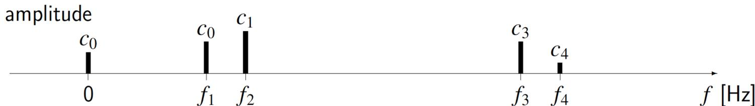
Formula:  $x(t) = c_0 + c_1 \cos(2\pi f_1 t) + \cdots + c_4 \cos(2\pi f_4 t)$
