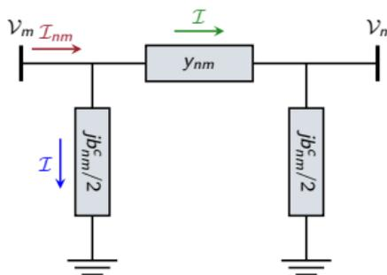
$$\begin{aligned} I_{nm} &= y_{nm} (V_n - V_m) + j \frac{b_{nm}^c}{2} V_n \\ &= \left( y_{nm} + j \frac{b_{nm}^c}{2} \right) V_n - y_{nm} V_m \end{aligned}$$
